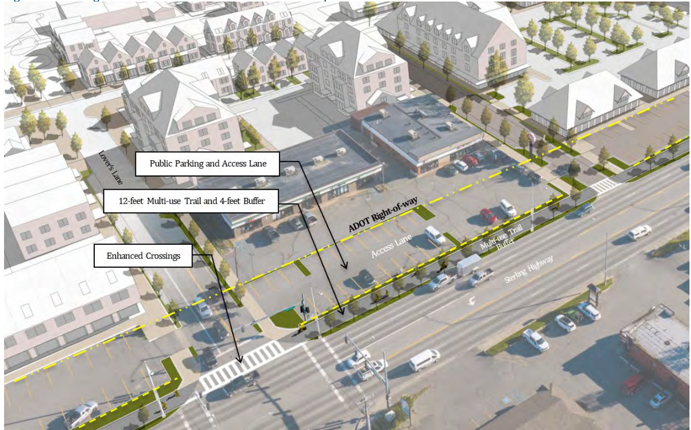
Figure 4: Parking Access Lane with Multi-Use Trail Concept
