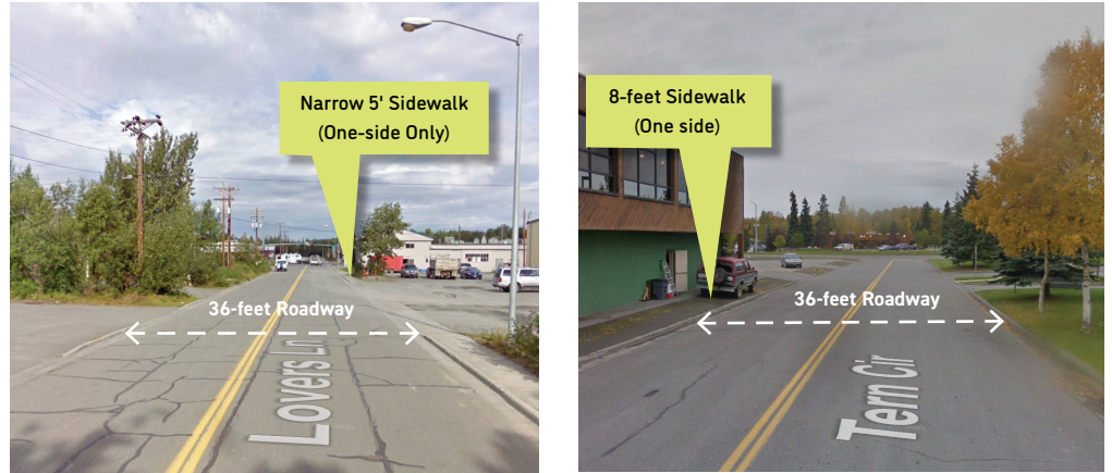
Fig. 75: Partially Improved Streets (Lover's Lane & Tern Circle)
